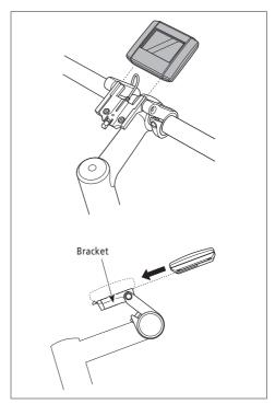
To remove the cycle computer, push the lever of the bracket firmly while sliding out the cycle computer.
